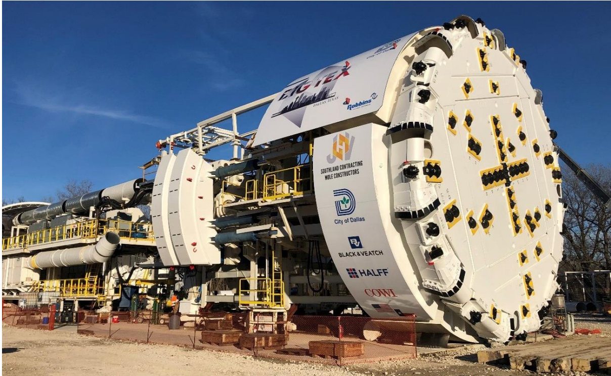
Figure 4-1 35ft diameter TBM at the Mill Creek Tunnel in Dallas, TX for flood protection.
